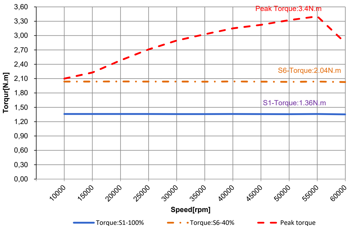
Torque Diagram (Cycle time:2 min)
